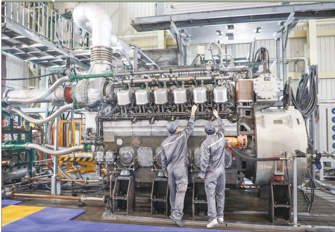
China's first medium-speed, high-power ammonia-fueled engine ignites successfully in Dalian, Northeast China's Liaoning Province, on November 30, 2023. This marks China's breakthrough and mastery of the key technology of ammonia-fueled engines. Photo: VCC
